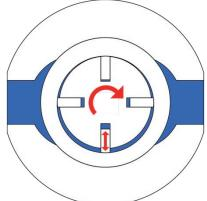
The pump housing is made of corrosion resistant solid block plastics like PP or PVDF. The motor power is transmitted by a frictional connection to the hydraulic part of the pumps by strong Neodynium-Permanent-Magnets. So the pump is able to work without any shaft seals, which guarantees a save and maintenance-free transfer of the liquid without any leakage of corrosive, toxic and explosive fluids.
