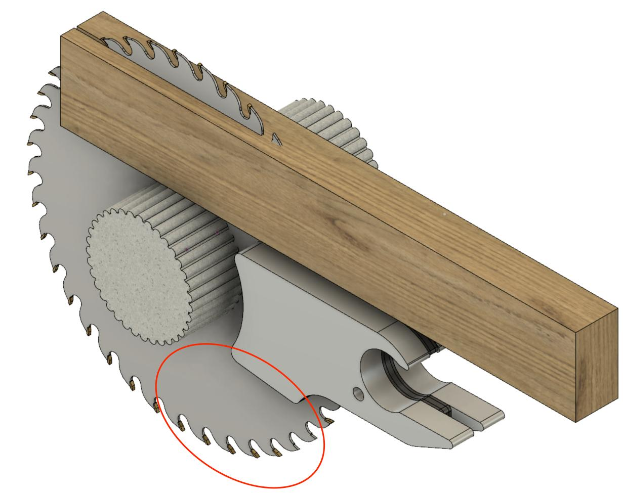
Safe area for placing a sensor
